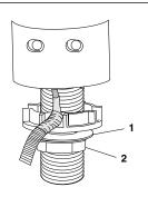
If faucet was installed with cover plate, secure cover plate with basin washers (1), flat washers (2) and locknuts (3).
